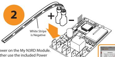
Power on the My N3RD Module. either use the included Power Supply or any other Power source with a voltage of 9-16 VDC (such as a car battery). If done correctly the "Power" LED should light up.
